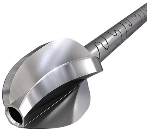
Fig 1 Flexible Monobloc Reamer with elastic shaft and deeply fluted reamer head incorporating both front- and side-cutting features to reduce intramedullary pressure, increase flow of bone chips and marrow, and facilitate high performance and efficiency.
