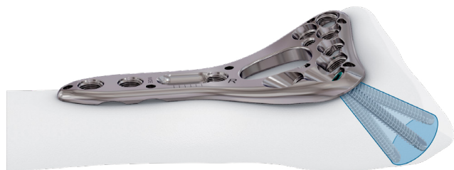
Fig 3 VOLT™ screw holes have a 30° cone of angulation with locking screws.
