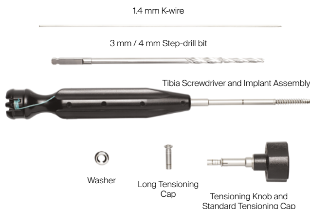
Fig 3 FIBULINK Syndesmosis Repair System components. The standard Fibula Tensioning Cap is preattached to the Tensioning Knob. The self-tapping Tibia Screw is preloaded to the Tibia Screwdriver. During drilling it is important that the larger diameter portion of the step-drill bit does not penetrate the tibial cortex.
